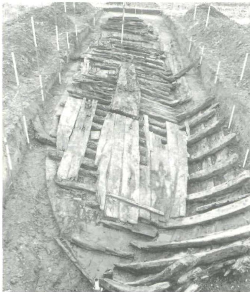
Figure 30. The hull with frames, mast step and ceiling planking.
